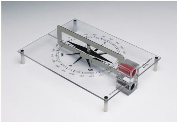
This apparatus demonstrates how an electric current affects a magnetic needle. The large transparent compass rose makes it possible to perform the experiment on an OHP.
