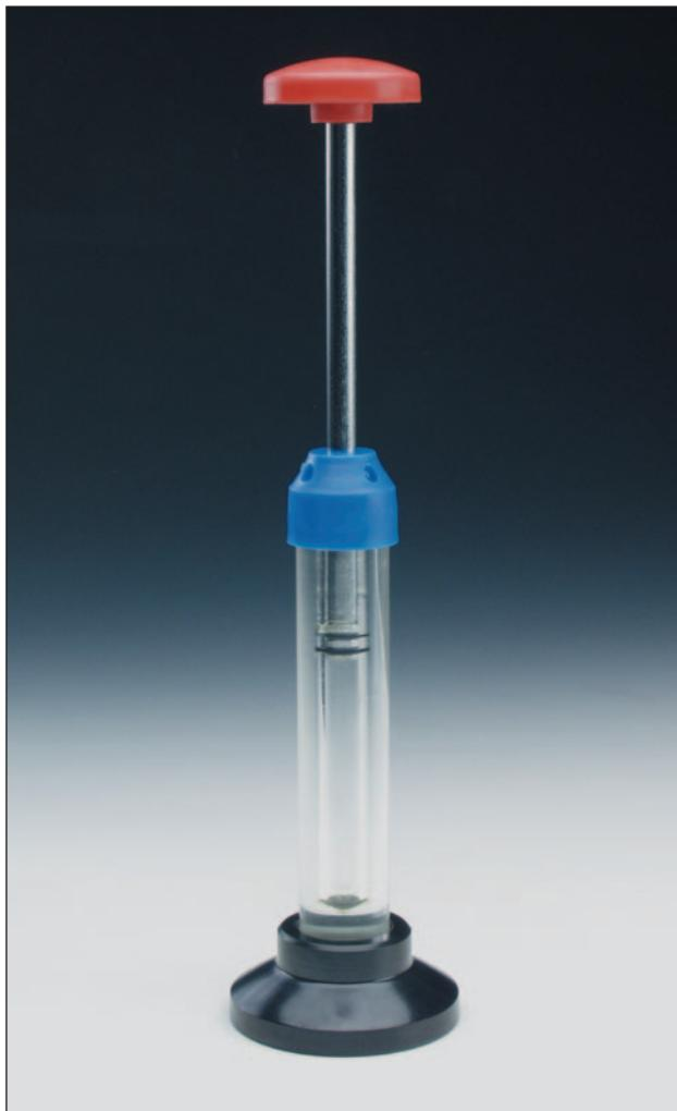
This equipment demonstrates that the temperature of a fixed mass of gas rises as the gas is compressed. If a piece of tinder is placed in the bottom of the cylinder, this will ignite when the piston is pushed vigorously down.
