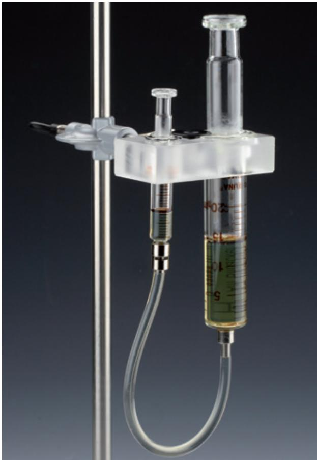
This model illustrates the working of the hydraulic lever: When the pistons are pressed down, a small force on the small piston will balance a large force on the large piston.
