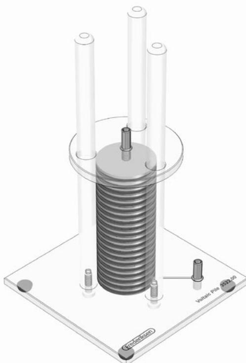
The voltaic pile is the first galvanic battery. Alessandro Volta invented the voltaic pile in the year 1800 made thereby possible the investigation of electric currents.
