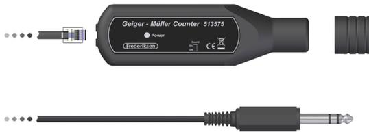
This Geiger-Müller sensor is suited for measuring alpha, beta and gamma radiation.
