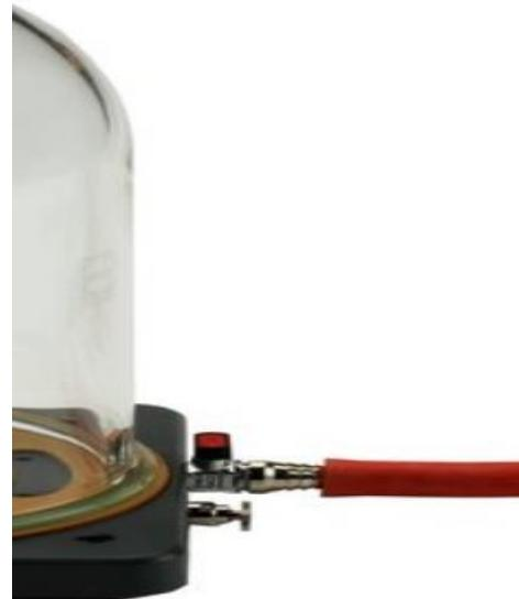
The pump plate is connected to a vacuum pump (069525) with a hose via a conical spigot with a diameter of 10 mm. The air in the bell is controlled with a valve tap and a thumbscrew for return air.
