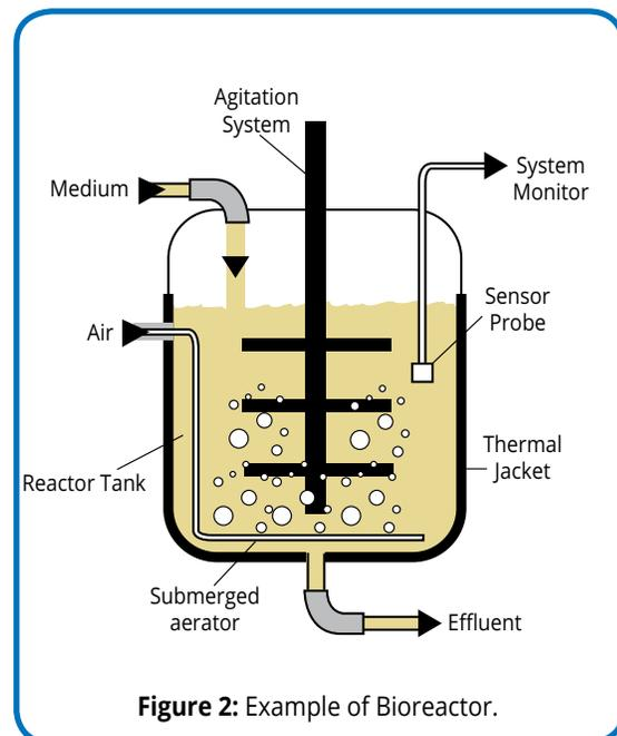
Figure 2: Example of Bioreactor.
