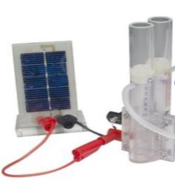
In the last step, the solar panel is connected to the electrolysis cell, as shown in the picture.
