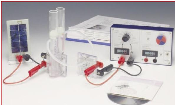
Complete energy set containing a solar cell which supplies electricity for the production of hydrogen, which is used by the fuel cell for the production of electricity. This current can be measured / displayed in the load box.
