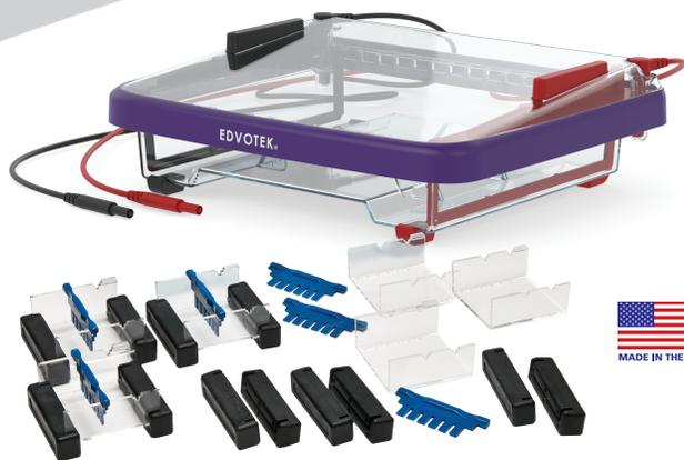
The newly redesigned M36 HexaGel™ electrophoresis apparatus has been engineered to yield excellent resolution in short periods of time! Each removable, UV transparent, E-Z Align™ tray features a molded embossing gel ruler and orientation arrow for the first sample. The M36 is ideal for student group experiments allowing the user to run up to six gels at one time.
